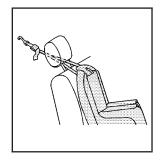
If the position you are using has an adjustable head restraint and you are using a dual tether route the tether under the head restraint and in between the head restraint posts. See *Head Restraints on page 13*.
